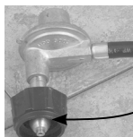
(B) Nipple has to be centered into the LP tank valve
