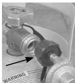
(C) Hold coupling nut and regulator as shown for proper connection to LP tank valve
