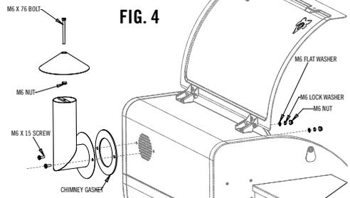
4. The height of the chimney cap can be adjusted for summer and winter. In the summer the gap should be approximately 1-1/2". In the winter the gap should be approximately 1/2".
