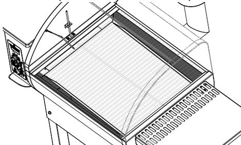
Direct heat will damage the meat probe wires. Always route the meat probes through ports on the side of the grill. Do not submerge wire in water. Not dishwasher safe.
