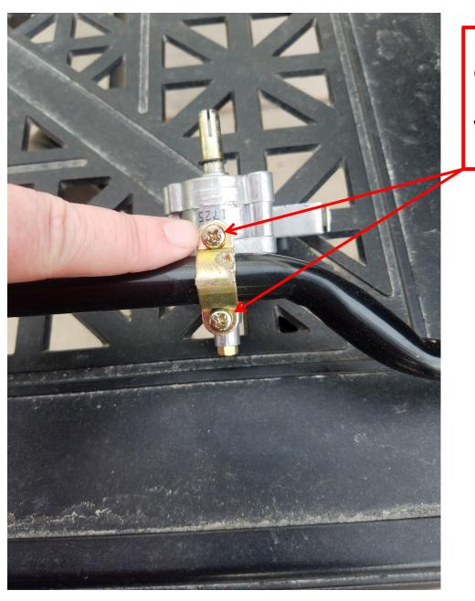
Once you have the manifold and valves disconnected from the face plate, you can remove the valve from the manifold. You will just need to remove these two screws from the connecting bracket
