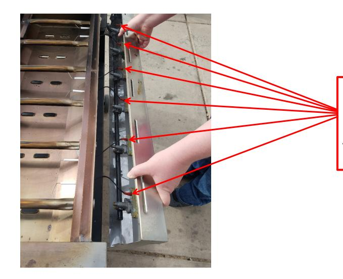
You will need to disconnect each igniter wire before you can pull off the cover that will house the manifold and valves.
