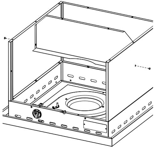
Install bottom assembly as shown using QTY 10 #10 screws. Note: Use a long Phillips screwdriver to reach through the access holes in the bottom assembly. You will need to reach through the large holes in the bottom to get the screws started.
