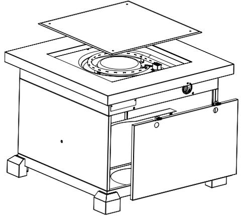
Install the 1/4-20 thumb screws to the door and secure in place with the 1/4 push nuts as shown. Make sure to insert the thumb screws from the outside as shown. The push nuts are pressed onto the threads of the thumb screw to hold in place.
