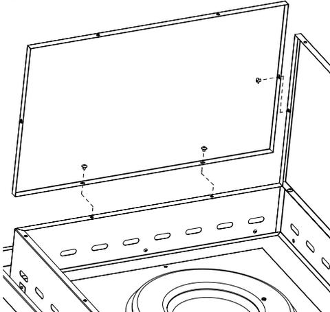
Install side panel as shown using QTY 4 #10 screws. Do not tighten the screws all the way at this point.
