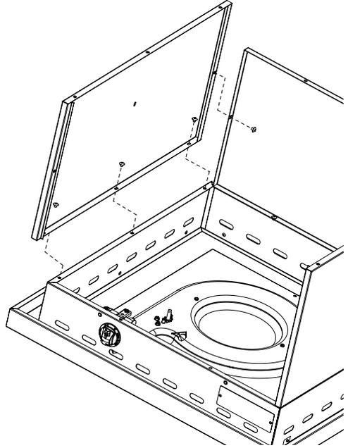
Install center panel as shown using QTY 2 #10 screws. Do not tighten screws all the way at this point. Note: Cutout for the tank should face the front as shown.
