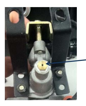
If you haven't assembled your smoker yet, remove the valve from the burner and use the specified drill to widen the valve's orifice.
